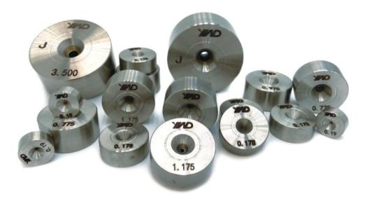
PCD wire drawing die is made of polycrystalline diamond material as drawing working area, through casing, drilling, lapping, polishing and other procedures to finish the die.
