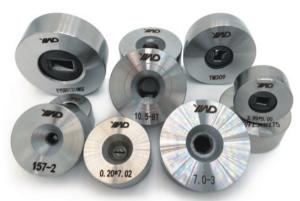
Shaped tungsten carbide wire drawing die is made of tungsten carbide as drawing working area, through shaped hole processing, lapping, polishing, casing and other procedures to finish the die.
