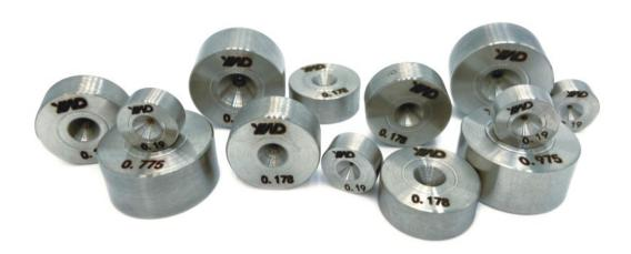
Single crystal diamond wire drawing die is made of natural or synthetic single crystal diamond as wire drawing working area, through casing, drilling, lapping, polishing and subsequent procedures to finish the die.
