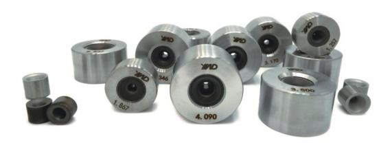
Nano diamond coated wire drawing die is a new type of wire drawing die, which is made of nanoscale diamond film on working surface(tungsten carbide base) of the die by chemical vapor deposition (CVD), through casing, lapping, polishing and subsequent procedures to finish the die.
