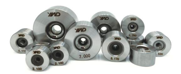
Tungsten carbide wire drawing die is made of tungsten carbide as drawing working area, through hole processing, lapping, polishing, casing and subsequent procedures to finish the die.
